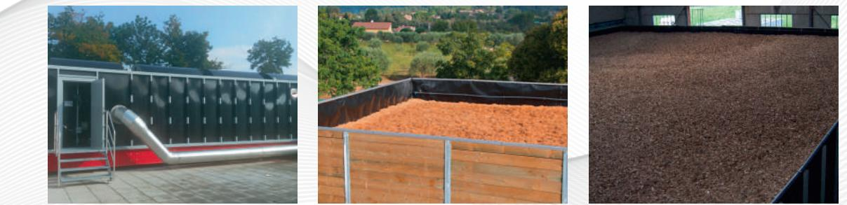
The nature of the biomass may vary depending on the type of pollutant to be treated. It is therefore possible to use bark of different wood species «chopped into chips of different sizes», coconut fibre, or fibrous peat.
